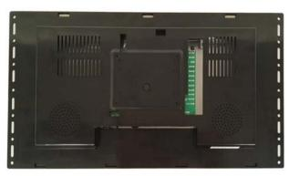
The 15.6" Openframe VideoPoster 1080P Media Player(ADOP-1560P) is a smart-designed video display, which can be easily integrated into a special housing, Kiosk, product display or any other type of product presentation. The frame is made out of plastic so it can be installed fully electronically isolated if requested. It has an extra inlet of power supply to support easy integration.
