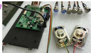
The 7" Openframe Media Player(OP7007-IPS) is a smart-designed video display, which can be easily integrated into existing chassis, Kiosk, product display, shelf-edge or any other type of product presentation. The frame is made out of metallic so it could be customized very easily with short lead time. It is also optional with motion sensor, push buttons, lift sensor, capacitive touch button, with built-in lighting distribution.
