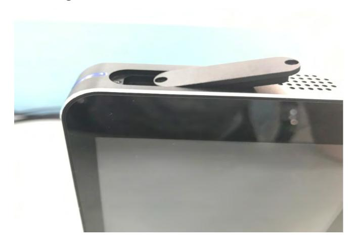
The bottom I/O door is specially designed via a separate tooling.
