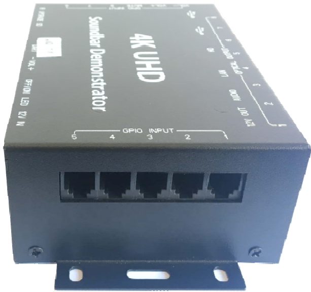
GPIO INPUT>>> Soundbar Selector Push Button With RJ11 Connector, from No.1 to No.5.
