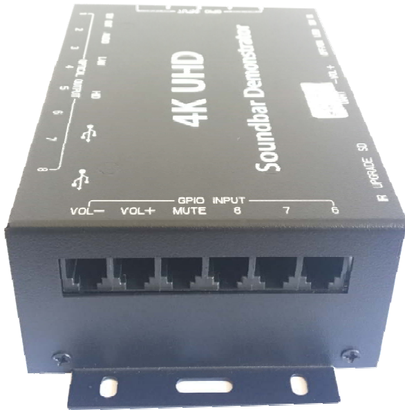
GPIO INPUT >>> Volume Control & Soundbar Selector Push Button With RJ11 Connector, From Left To Right: Volume Down, Volume Up, Mute, No. 8 Soundbar, No.7 Soundbar, No.6 Soundbar
