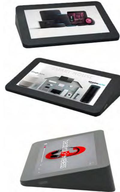
An industrial grade 15.6-inch touchscreen monitor working with Brightsign media player via I/O Ports of digital/analogue audio, GPIO, serial to control LED lighting, video, user interactivity
