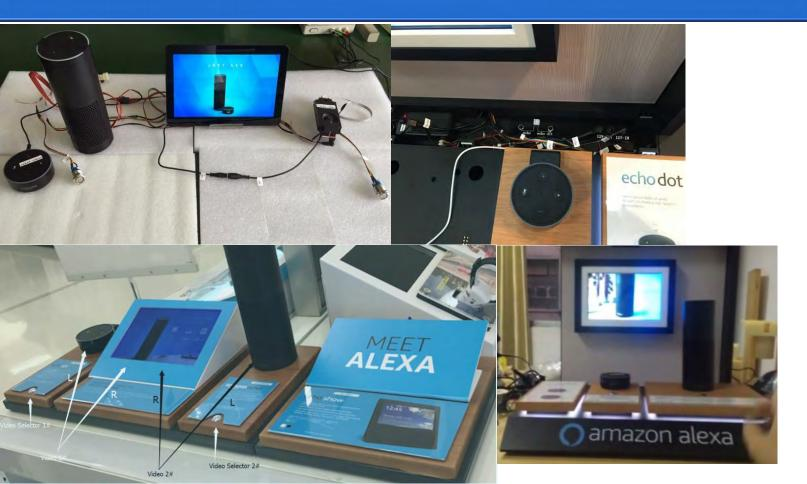
By separating L & R channel of the audio of Amazon echo retail ads video, the retail station simulates the real user scenario when amazon echo speakers are connected. The introduction audio is sent to the public speaker, while the echo bot audio are sent to the designated echo speaker to help user visualize and experience the real application.
