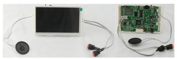
The 7" Openframe Media Player (OP7002DP) is a smart-designed video display, which can be easily integrated into existing chassis, Kiosk, product display, shelf-edge or any other type of product presentation. The frame is made out of plastic so it can be integrated into any fixtures with safety. It is also optional with motion sensor, push buttons, lift sensor, capacitive touch button, with built-in lighting distribution.
