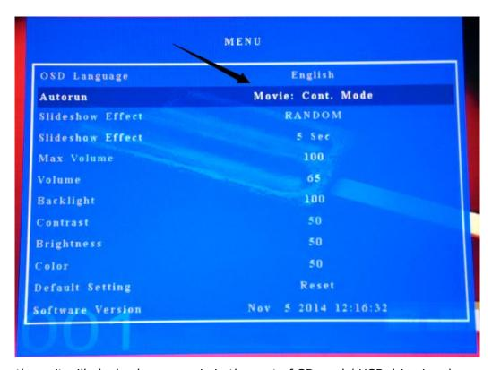
In this mode, the unit will playback any movie in the root of SD card / USB drive in a loop.
