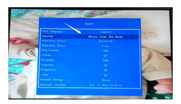
In this mode, the unit will power on to loop the default video named mu.avi, and the movies 00.avi, 01.avi, 02.avi, 03.avi could be activated via push buttons which are connected to the GPIO controls labeled LED00, LED01, LED03.
