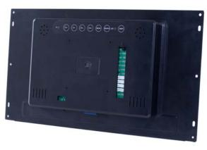
The 13.3" Openframe VideoPoster 1080P Media Player(OP1331) is a smart-designed video display, which can be easily integrated into a special housing, Kiosk, product display or any other type of product presentation. The frame is made out of plastic so it can be installed fully electronically isolated if requested. It has an extra inlet of power supply to support easy integration.
