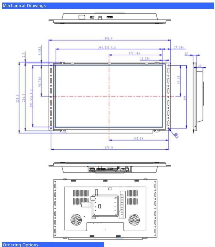
Player Console: 15.6 inch openframe video player AC Adatper: 12V /1A Push Button: 5V LED Plastic / Metallic Motion Sensor: 120 degrees / 1.8 Meters Touchscreen: 4-Wire Resistive
