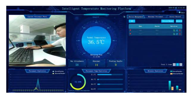
LAN application is used to demonstrate the traffic conditions of personnel, support the real-time display of traffic records, device management, data export, abnormal temperature handling and other functions.
