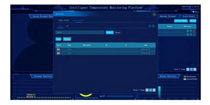
Send the personnel information of the current device to another device: select the device and click "Send" button to check the device that needs to be synchronized, and click "Confirm" to conduct the operation of sending personnel information.
