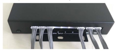
Connect Push buttons in GPIO 1#,2#,3#,7#, and V+, V-
