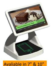
The 7" Android Kiosk(ADPOS-701) is a smartdesigned self-serivce kiosk for entertainment, ordering, menu display as well as pay-at-table with RFID reader as well as interface for integration into customer's existing POS infrastructure. With its interactive capabilities, customers can easily customize their own kiosk with app to tailor-made solutions.
