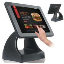
The 9.7" Android Kiosk is a smart-designed self-serivce kiosk for entertainment, ordering, menu display as well as pay-at-table with RFID reader (optional) as well as interface for integration into customer's existing POS infrastructure. With its interactive capabilities, customers can easily customize their own kiosk with app to tailor-made solutions.
