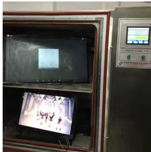
Reliability Verification: Aging @ -20°C - 60°C for 72 hours
