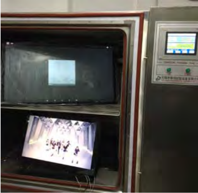
Reliability Verification: Aging @ -20^{\circ}\text{C} - 60^{\circ}\text{C} for 72 hour
