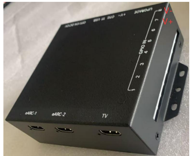
7# button for V+, 8# button for V-
