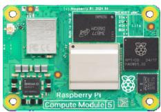
Compute Module 5 is a powerful and scalable system on module with a 64-bit Arm processor @ 2.4GHz, an I/O controller, video and PCIe interfaces, and a range of wireless, SDRAM and eMMC options. Developers can leverage its efficient software stack in their own embedded systems, with our I/O extension board and expertise in LCD screen & touch panel, they can quickly have their ready to ship smart hardware, manageable, scalable and fully under their own control.
